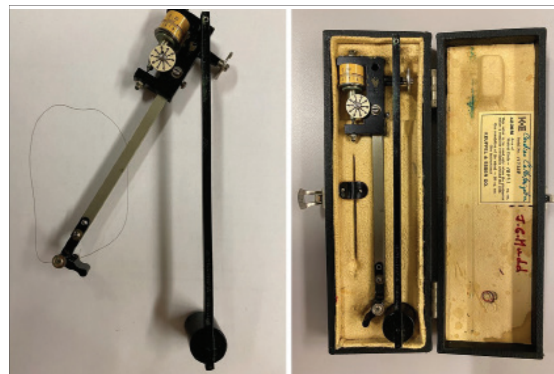
FIGURE 4. Mechanical hand planimeter, circa 1965, used for calculating planar areas on paper tracings. The numbered wheels at the top move as the arm traces the area, adding positive values in one direction and reducing them as the arm moves back, producing a net area in square centimeters. A standard circle with known area was originally provided for calibration, but has been lost. Technology replaced hand planimetry about 40 years ago.
